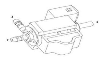
3. Using clean shop air regulated to 80-100 PSI (551-689 kPa), blow through all three ports (1, 2 &3) for 5 seconds each. Repeat this step twice.
