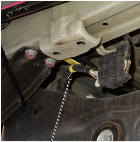
REAR SUBFRAME HARNESS Disconnect.
