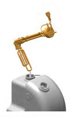
48 Remove the retaining clip (1).
