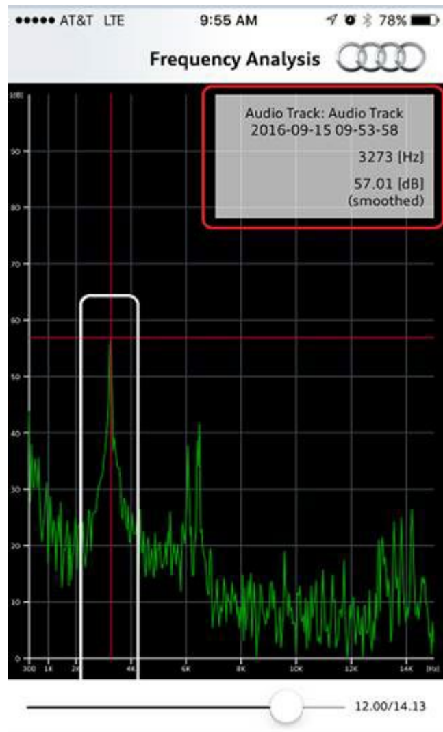
Figure 6. Typical brake squeal frequency recording.
