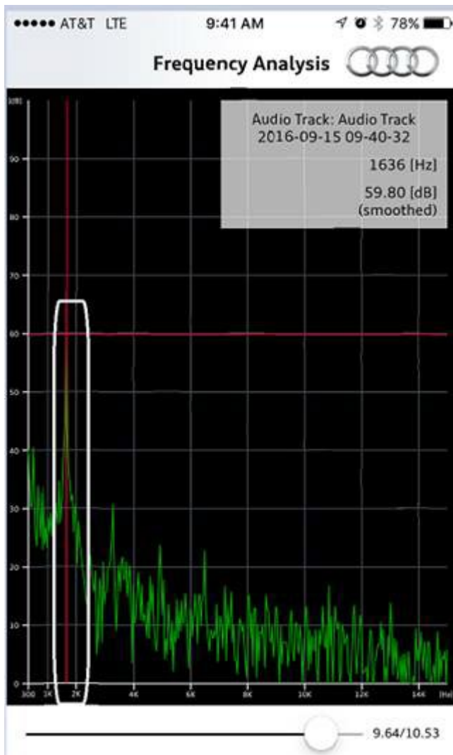
Figure 5. Other sounds can disguise the main frequency.
