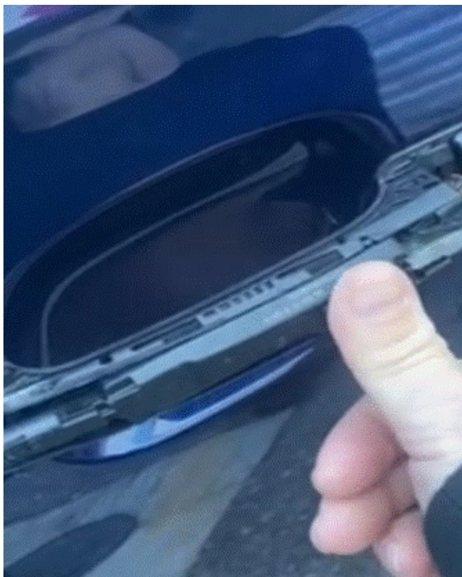
Figure 4. Activating the locking system touch sensor with door handle trim plate removed.
