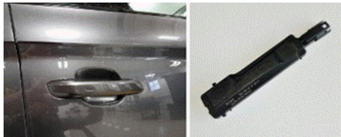
Figure 1. Outer door handle and keyless locking touch sensor.
