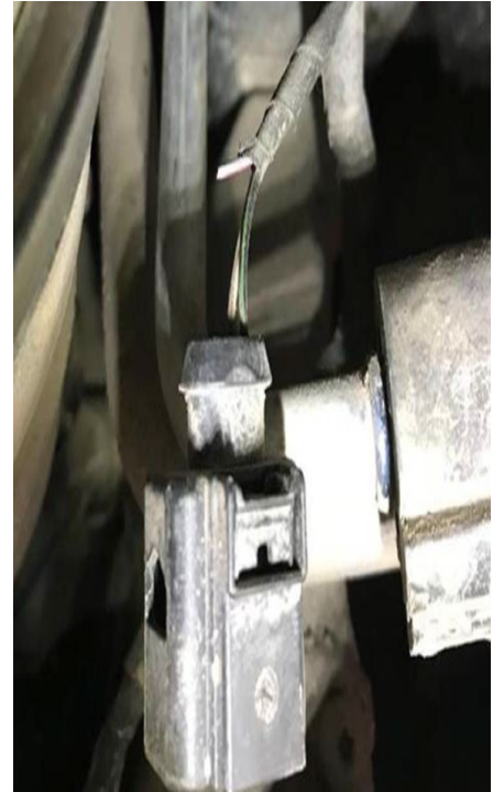
Figure 1. N280 control wire damaged at T3r connection
