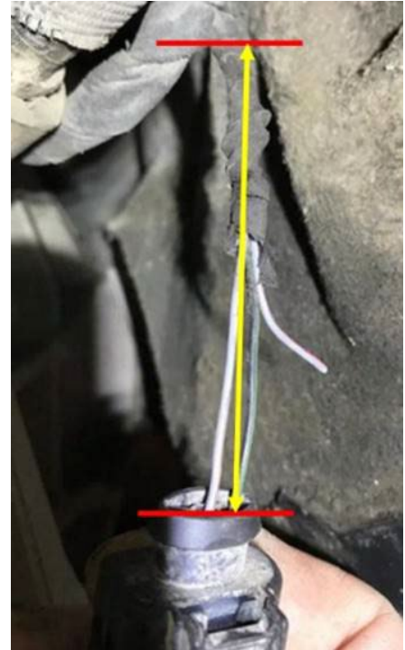
Figure 2. Measure 110 mm from T3r to the first harness branch
