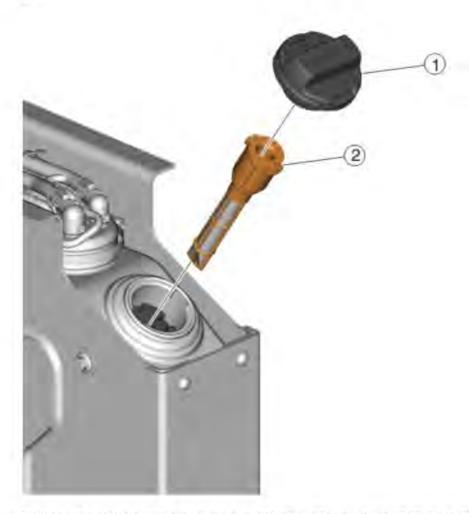
Release the retaining tabs and remove defective filler neck insert (2) from DEF tank.
