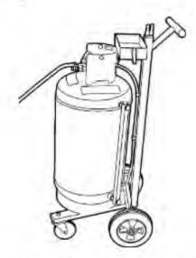
Connect the coolant extractor to the drain fitting at the bottom of the radiator and drain the coolant.
