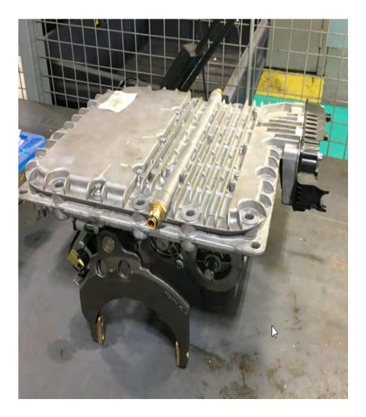
The 2/3 and the 1/R shifter have a shift detent between them similar to a regular manual gearbox will have to prevent shifting into two gears at one time. If either of these shifters will not move when shifting manually then check the other shifter and verify that it is in the neutral position.
