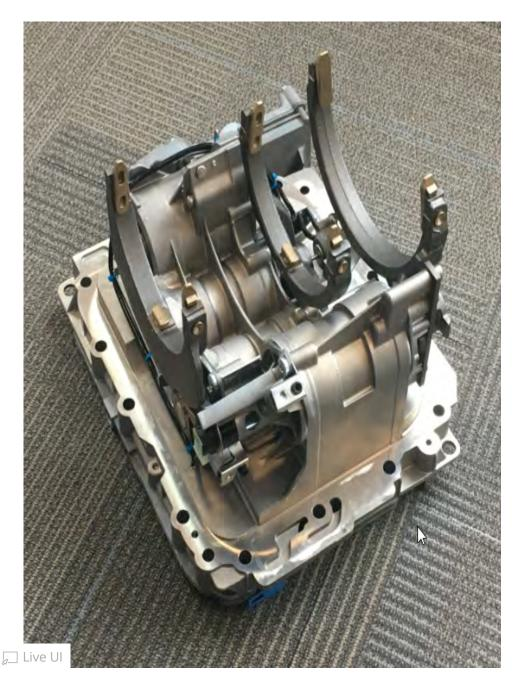
For automated testing using Tech Tool rest the shift housing on its forks on a flat smooth surface.
