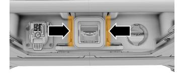
6. On both sides: Insert a shim or similar tool through the gap(s) between the trailer hitch and closeout panel. Use the tool to push the harness off of the bracket so that it is not trapped.
