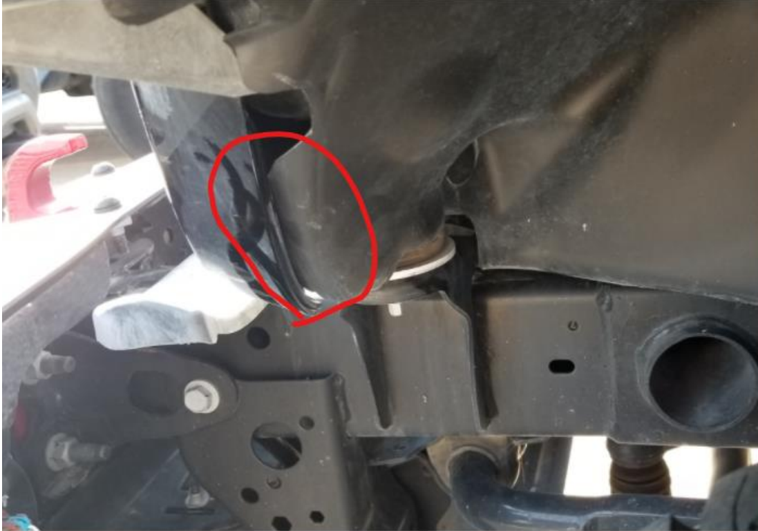
Properly tucked wheel liner. Flap is behind grille.
