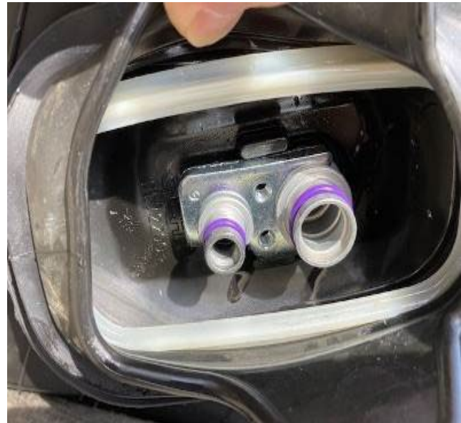
Figure 3. Refrigerant connections to the expansion valve.
