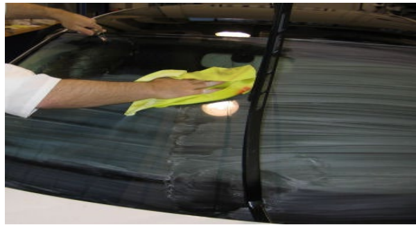
Figure 7. Rinsing the windshield.
