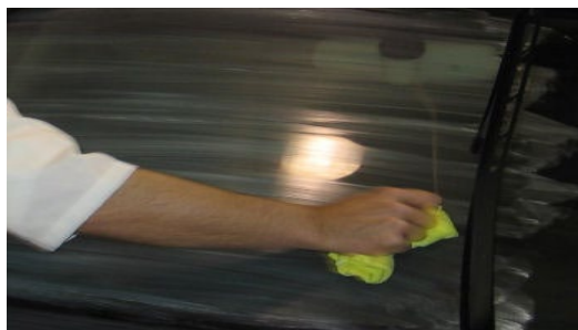
Figure 6. Using horizontal strokes to clean the windshield.
