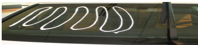
Figure 4. Cleaner applied to the windshield.
