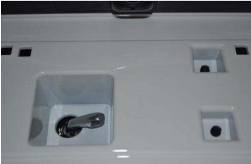
Remove the key shank from the key fob, insert it into the lock cylinder, and rotate. This should mechanically release the rear hatch / rear compartment. If access is still not gained through the back up mechanical method, see the section later in this document titled, "Accessing the rear hatch / rear compartment with a seized up latch."
