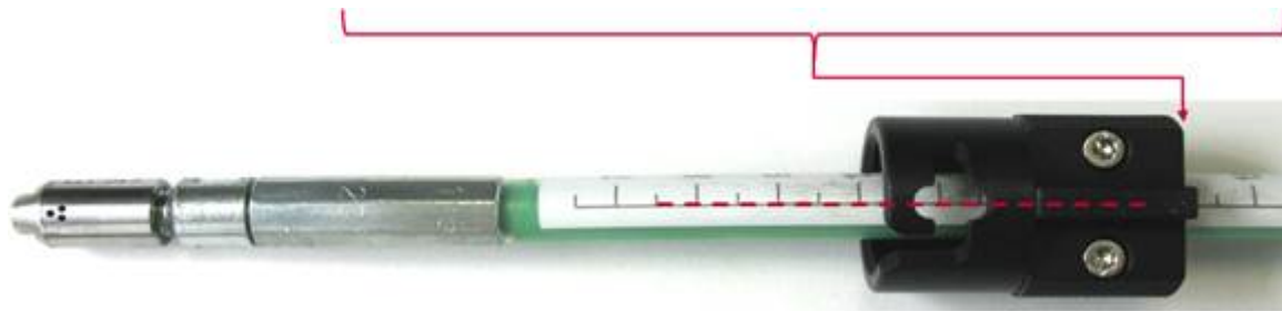
Figure 12: Arrow indicating how the back side of the adaptor must align with the scale. Red dotted line indicating how the longitudinal slot must align with the black line on the scale.
