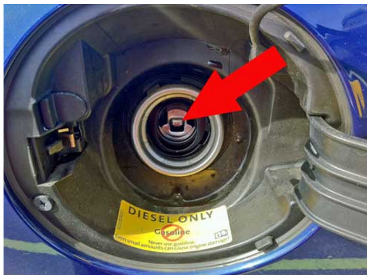
Figure 1. Misfueling guard, indicated by red arrow. (2013 A3 TDI pictured. Other vehicles may appear slightly different.)
