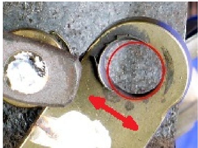
Figure 1. Worn eye on wastegate link plate allowing excessive play.
