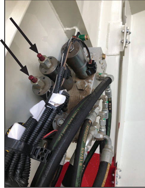
This side view shows the valve overrides (red buttons at the end of the cartridge).
