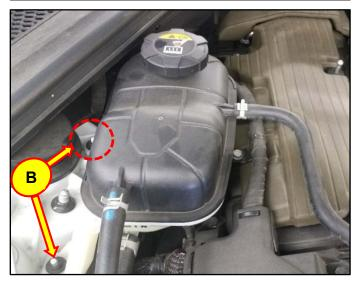
TSB #: 22-01-060G Page 2 of 5 4. Remove the radiator reservoir tank (C).
