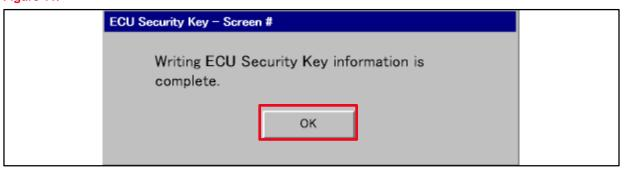
9. Confirm the ECU security key has been properly written by performing a Health Check and confirming the ECU security key indicator shows "-", and then clear ALL DTCs.
