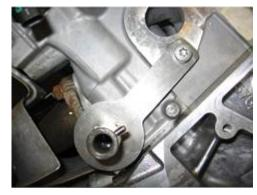
Figure 10. Engine adaptor on bank one.
