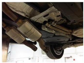
Figure 4. Lowered catalytic converter pipes
