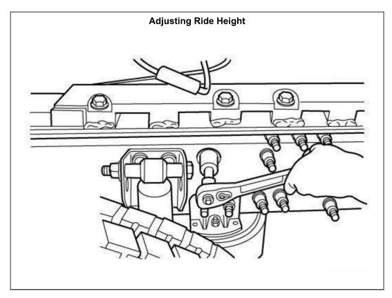
To adjust ride height, loosen the height control valve bracket mounting bolt so that the bracket is free to pivot about the bolt, then insert the adjustment tool through the access hole in the frame rail. Rotate the height control valve and bracket clockwise to raise, or counterclockwise to lower ride height. After proper ride height has been achieved, tighten the height control valve bracket mounting bolt to 50 N•m (37 lb-ft).
