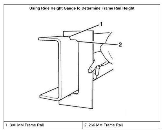
After determining frame rail height, measure chassis ride height as outline in the instructions on the gauge. Ride height is correct when the "ACCEPTABLE RANGE" marks (for the frame rail height being serviced) align with the bottom edge of the air spring mounting flange.
