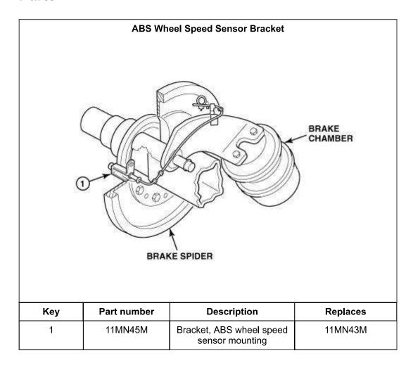
Note: If contact between the wheel speed sensor mounting bracket and tone wheel has occurred, inspect the tone wheel for damage and replace as required.
