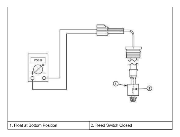
If sensor resistance is not within specifications, replace the sensor.
