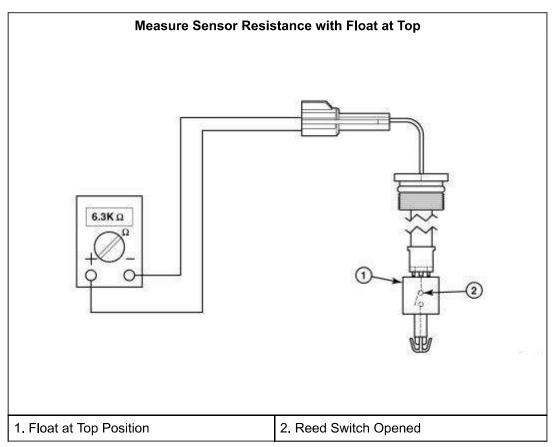
4. Move the float to the bottom of the sensor. At the bottom position, the reed switch should close, and the meter should indicate 750 ohms.
