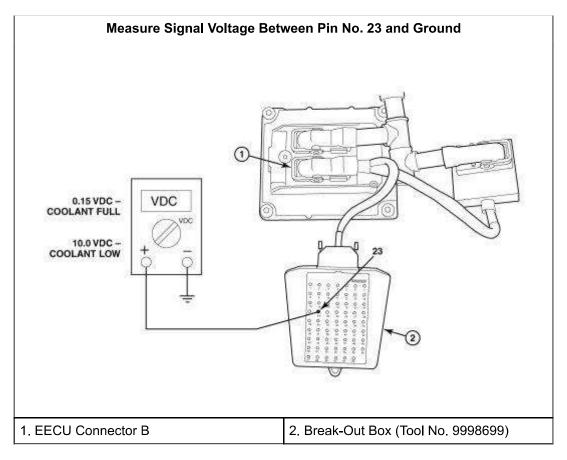
8. Drain enough coolant from the cooling system to bring the level of coolant below the level of the coolant level sensor and note the voltage indicated on the multimeter. With the level of coolant below the sensor, signal voltage should be 10 VDC.
