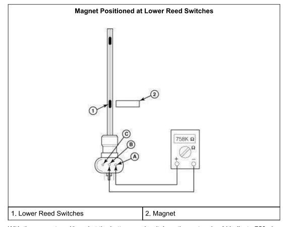
With the magnet positioned at the bottom reed switches, the meter should indicate 758 ohms.
