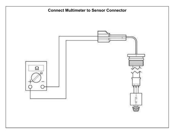
3. Hold the sensor float at the top position and note the reading indicated on the meter. Resistance should be 6,300 ohms.
