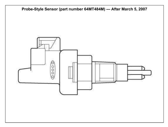
The probe-style coolant level sensor was implemented into production on CXP and CTP models equipped with US04 emission-compliant MP7 engines beginning March 5, 2007. This sensor utilizes a three-pin connector, whereas the previous float-style sensor utilized a two-pin connector.
