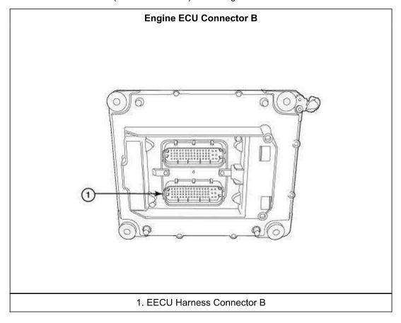
7. Turn the ignition key switch to the ON position, and then use a digital multimeter to measure signal voltage at pin 23 of connector B and a good ground. Signal voltage should be 0.15 VDC or less with the coolant at the specified level in the surge tank.
