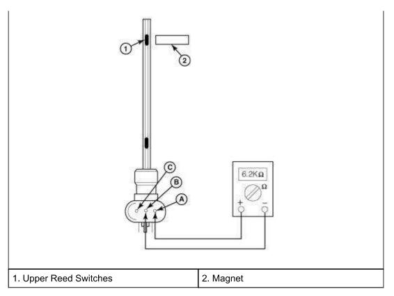
With the magnet positioned at the upper reed switches, the meter should indicate 6,220 ohms.
