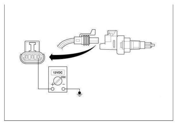
If 12 VDC is not present, check the 5 amp fuse in the external fuse holder (secured to terminal No. 1 of the 10-post trailer terminal strip). If the 5 amp fuse is OK, look for an open in the wire between terminal No. 7 of the 10-post trailer terminal strip and the coolant level sensor connector.
