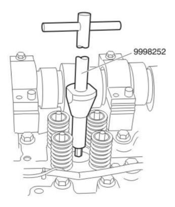
Install tap holder in the engine injector bore. Apply moderate downward force to get the tap started while turning the tap handle clockwise. Continue turning in the same direction, without reversing, until the copper sleeve is tapped all the way through. The shoulder of the tap handle bottoms on the copper sleeve. Ensure that the tap is completely through the copper sleeve
