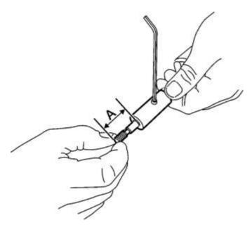
Install the extractor bolt into the end of the extractor tool. Adjust the bolt until it extends approximately 22 mm (0.9 inch) beyond the end of the tool (dimension A).
