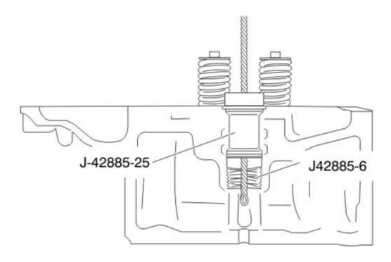
Using the brush, clean the cylinder head injector bore walls for the injector sleeve.
