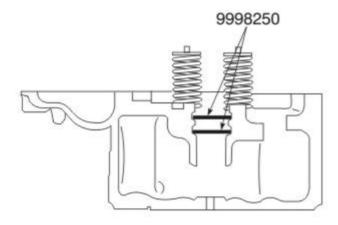
Install two sealing rings to prevent dirt from entering the fuel gallery when the copper sleeve is removed.
