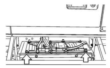
Install all previously removed cables to the ground (negative) battery terminals.
