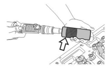
Install the protective sleeve over the engine injector to prevent damage.
