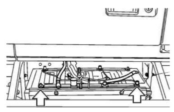
Disconnect all cables from the negative (ground) battery terminals to prevent personal injury from electrical shock and prevent damage to electrical components.
