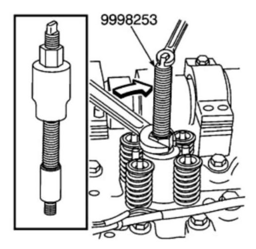
While holding the top of the tool stationary, turn the large nut clockwise to extract the copper sleeve.
