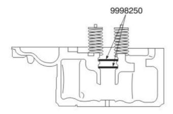
Attach a small diameter air line to a wet / dry shop vacuum nozzle that can reach into the coolant passages in the injector sleeve bore. Remove all remaining fuel and coolant. A lint free paper shop towel can also be used to absorb liquid. All fluids must be completely removed before proceeding. Remove the two sealing rings from the fuel passage when all fluid has been removed.
