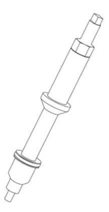
Place the new copper sleeve on the sleeve installation tool.
