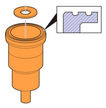
Before installing the copper sleeve, inspect it to ensure that it is the correct part. The correct sleeve is identified by two concentric circular grooves machined into the top surface.
