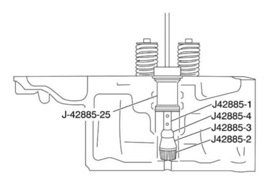
Using the cleaning kit, clean the injector sleeve seat of the cylinder head.
