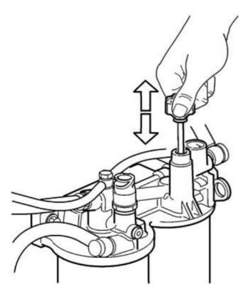
Prime the fuel system by pumping the hand priming pump on the fuel filter housing until resistance is felt indicating that the system is full of fuel.
