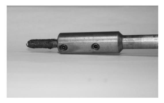
Completely coat the 8.5 mm tap with fresh, extreme pressure NLGI #2 grease or equivalent.
