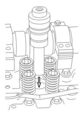
Clean the protective plug and install it into the injector bore of the cylinder head to protect it from debris. Using compressed air, clean out the injector hold down bolt holes.
