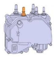
• If the system is able to build pressure: The pump in not the issue. Further diagnosis is needed for the supply side of the system. Inspect the below components and repair as necessary:
