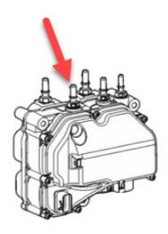
**3.** Connect a clear 3/8" (inner diameter) hose to the fitting and place the other end of the hose into the DEF Tank.
