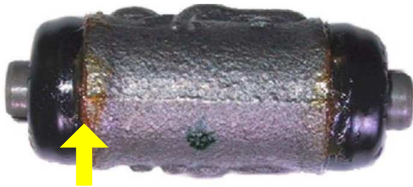
There may be bleeding of the rust prevention grease.
