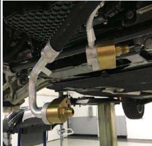
Figure 6. Installation of VAS 6338/3 and 6338/12.
