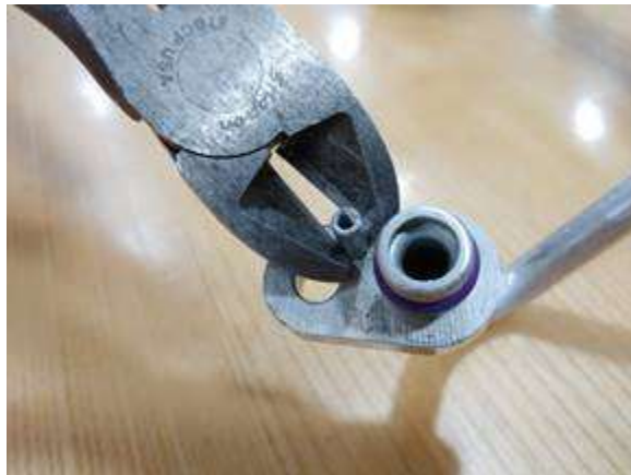
Figure 15. Removal of dowel pin.
