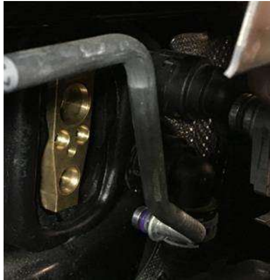
Figure 3. Installation of front expansion valve bypass adaptor VAS 6338/38.
