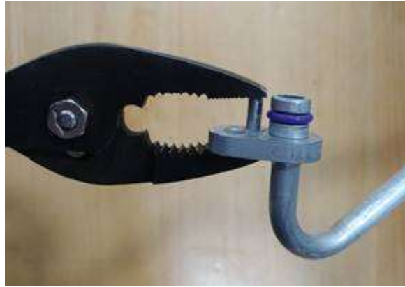
Figure 16. Installation of rear refrigerant line dowel pin.
