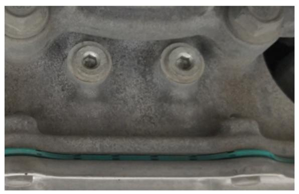
Remove the suspect plug, discard and clean the threaded hole with a clean lint free shop towel to remove residual oil.
