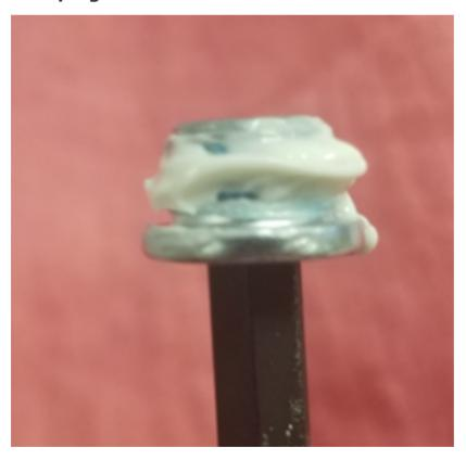
Install the new plugs torquing to 11 lb ft (15 Nm) and clean the area around the plug.
