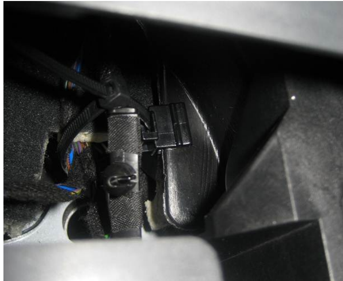
Figure 9. Zip tie needs tightening.
