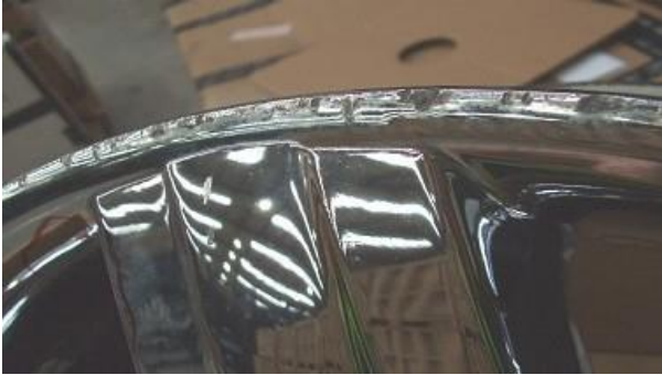
Figure 8 Damage to the rim due to curbing but also damage to the spoke caused by impact damage, such as stone chips
