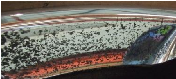
Figure 9 Pitting is not a manufacturing defect and cannot be claimed under Warranty (Figure
