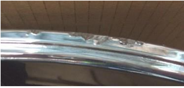
Figure 7 Marks on the rim due to curbing
