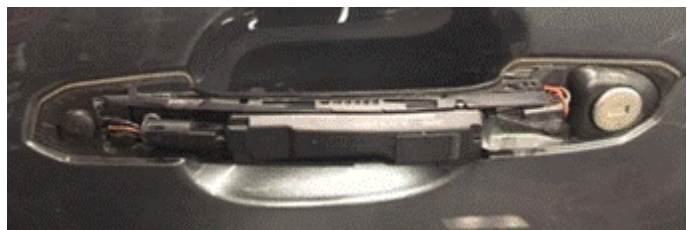
Figure 3. Exposed locking system touch sensor with door handle trim plate removed.
