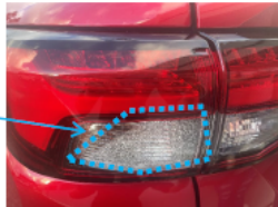
Outlander rear taillight with dew condensation
