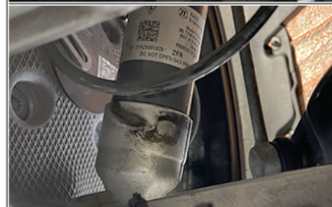
Traces of oil on rear axle shock absorber
