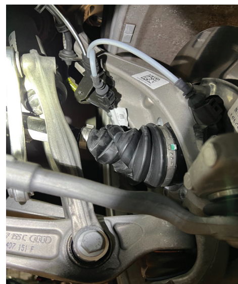
Figure 1- Driveshaft detached from splines at outer joint
