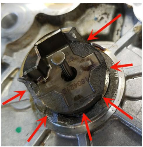
Rotate the exhaust camshaft to position the 2D matrix marking on the camshaft hex in the 12' O'clock position. (Reference photo below for 2D marking.)
