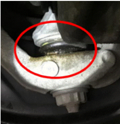
Figure 1: Grease emerging from swivel joint.
