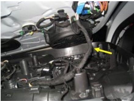
Figure 12. Wire harness not secured properly.
