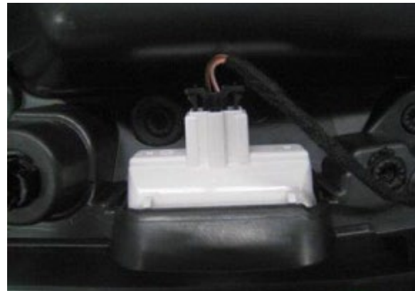
Figure 17. Wrapping light wire harness with fleece tape.
