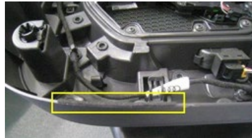
Figure 15. Felt tape installed on trim panel.
