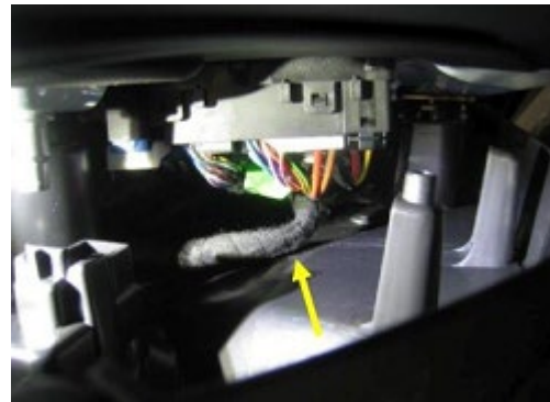
Figure 11. Wire harness contacting door trim panel.
