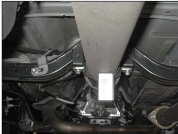
Figure 11. CORRECT Placement of Digital Angle Gauge
