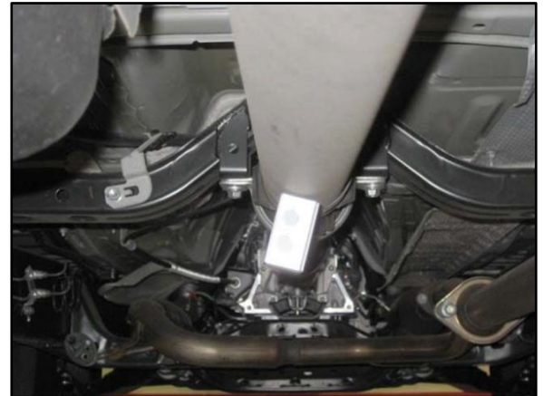
Figure 12. INCORRECT Placement of Digital Angle Gauge
