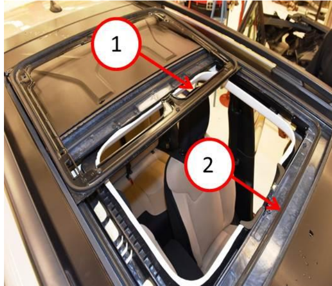
Fig. 5 Frame And Primary Seal
