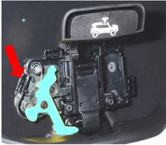
Fig. 9 Cover Handle Clip With New Lever
