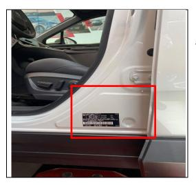
a. Open Driver Side Door and Locate Lower B Pillar
