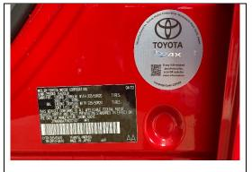
b. Wipe location with cleaner to ensure adhesiveness c. Install label on Lower B Pillar as shown.
