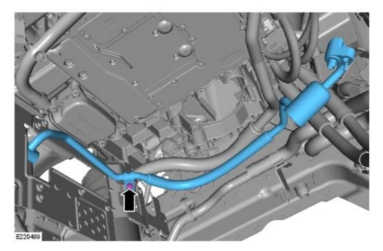
Remove the <u>A/C</u> compressor HP pipe.
