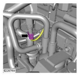
Disconnect the electrical connector from the  $\underline{A/C}$  temperature and pressure sensor.
