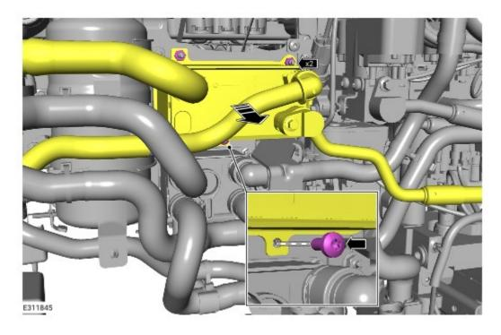
Reposition the indirect condenser away from the bracket.
