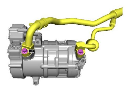
Disconnect both <u>A/C</u> pipes from the <u>A/C</u> compressor.
