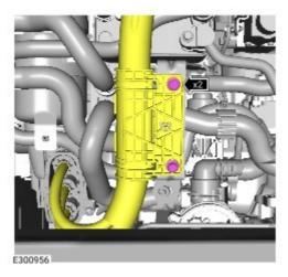
Reposition the High Voltage (HV) harness away from the bracket.
