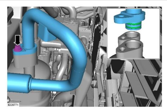
Disconnect the  $\underline{A/C}$  compressor LP inlet pipe from the accumulator and remove the pipe.
