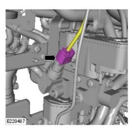
Disconnect the electrical connector from the  $\underline{A/C}$  HP temperature sensor.
