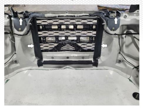
**3.** Relocate the wiring harness by removing the harness retainer clips to allow the harness to lie on the top of the hood.
