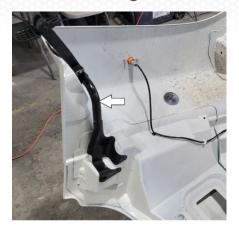
21. Reinstall the left and right rubber baffles from the inner grille
