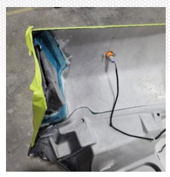
**9.** Use paper to cover inside of the grille to protect the grille from resin drips.
