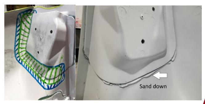
Clean all sanded areas by blowing off all dust and using a tack cloth to remove all fine dust particles.
