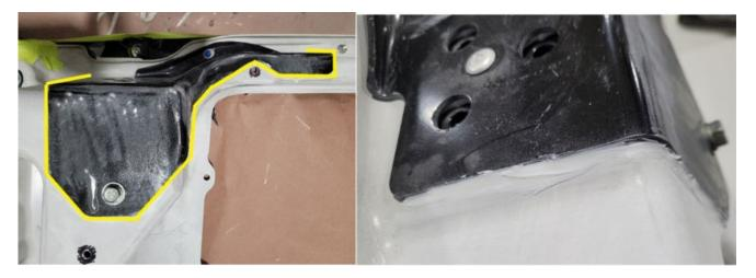
If necessary, use Loctite Power Grab heavy duty construction adhesive (or similar) at the joint between the hood support bracket mount and the hood.
