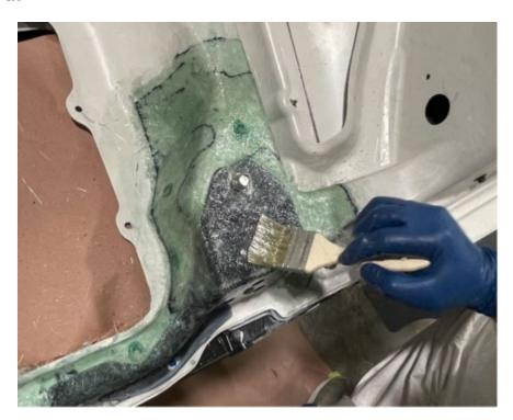
Repeat the process for each additional sheet of fiberglass.
