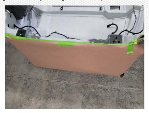
**11.** Mark with a permanent pen all wire harness retaining clip holes that will be covered with fiberglass. There are 4 holes to mark on each side of the hood.
