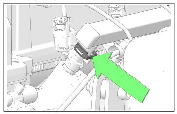
9. Using soap and water, clean the surface of the old quantity label. Install the NEW oil quantity label, supplied in the kit, over the existing label as shown.
