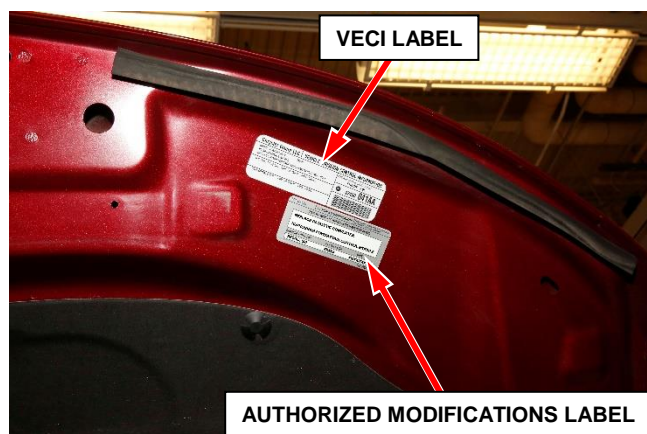
Figure 12 – Apply Authorized Modifications Label Near VECI Label (Specific Vehicle May Look Different)
