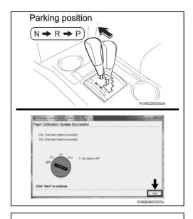
After "Flash Calibration Update Successful" is displayed, move the shift lever to Parking position and turn the IG off and click the "Next" button.
