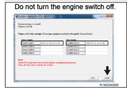
After "Flash Calibration Update Successful" is displayed, move the shift lever to Parking position and turn the IG off and click the "Next" button.
