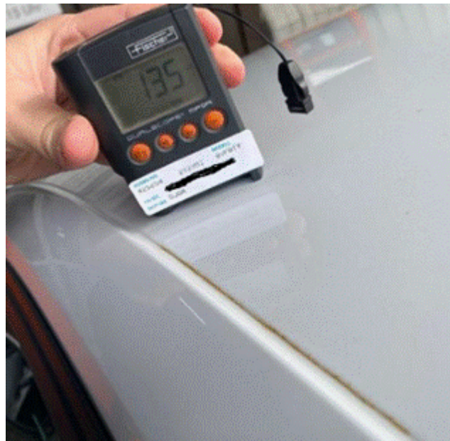
Figure 6. Paint thickness measurements.
