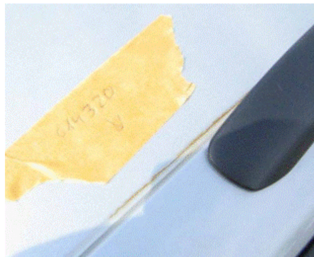
Figure 1. Resultant corrosion due to cracks in the paint.
