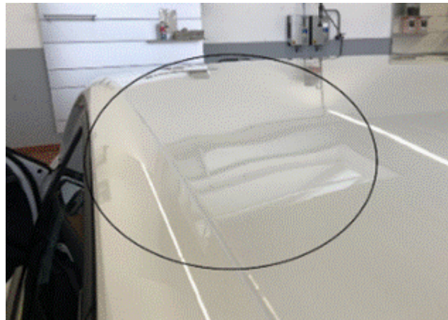
Figure 4. The remaining roof deformation may evade a brief view of the roof panel.
