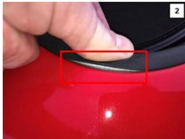
Figure 2. Checking the adhesion quality.
