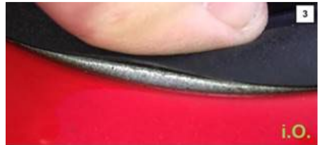
Figure 3. A properly adhered perimeter seal.
