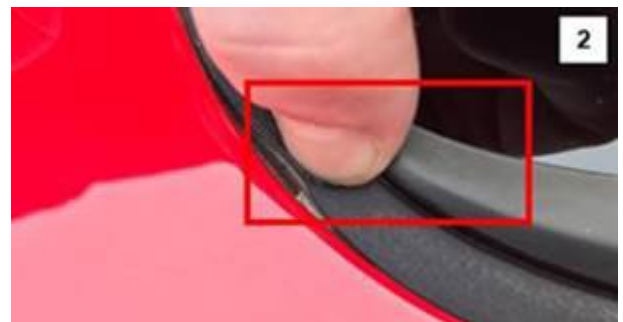
Figure 5. Clear evidence of adhesive detachment.
