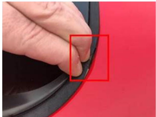
Figure 7. Adhesive band detachment.
