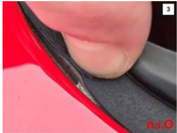
Figure 6. Seal adhesive band detachment revealed.
