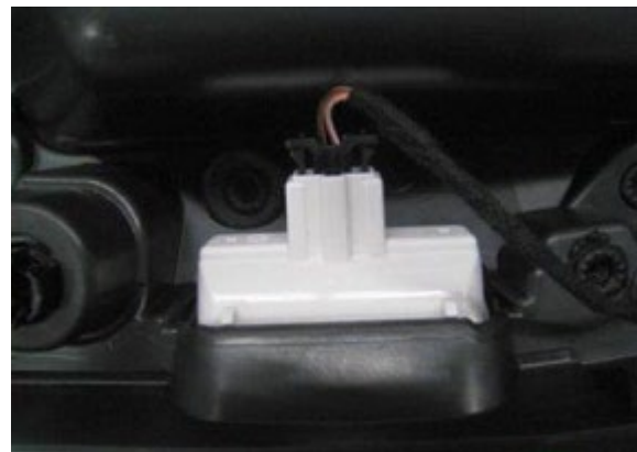
Figure 17: Wrapping light wire harness with fleece tape.
