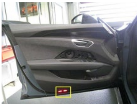
Figure 16: Apply fleece tape to trim panel light and wiring.
