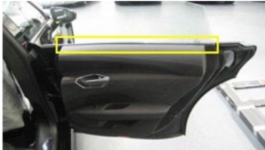
Figure 3. Apply fleece tape to the trim panel mounting strip.
