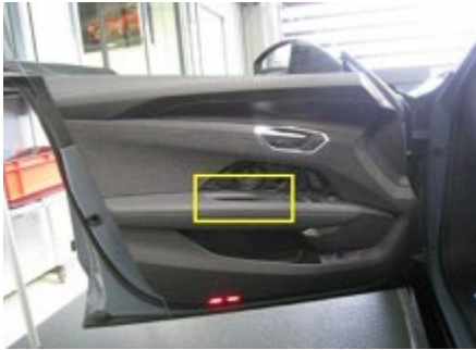
Figure 8. Isolate pull handle from armrest.
