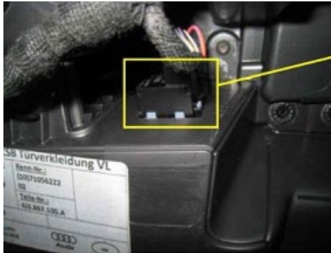
Figure 21. Apply fleece tape to pocket lighting.
