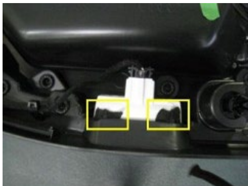
Figure 16: Apply fleece tape to trim panel light and wiring.
