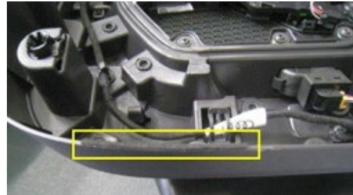
Figure 15: Felt tape installed on trim panel.
