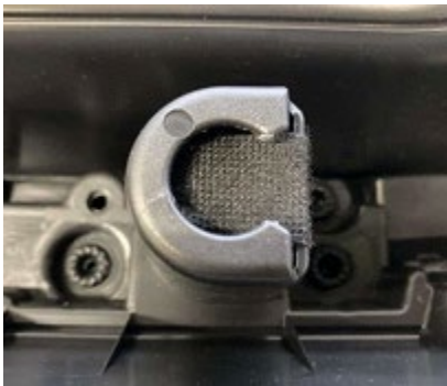
Figure 6. Door clip with fleece tape applied.
