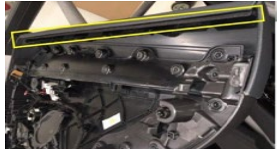
Figure 4. Fleece tape applied to mounting strip.
