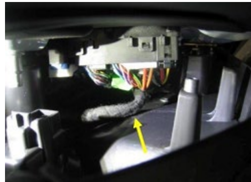
Figure 11. Wire harness contacting door trim panel.
