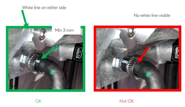
3) If both retaining clips are OK, no further work is required.
