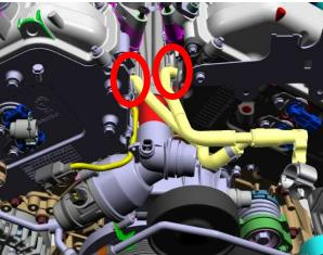
2) Using an endoscope, check if the retaining clips (jubilee clips) are secured in the correct position. The hose should be fitted closely to the mating part and the retaining clip (jubilee clip) should be positioned with white marks being visible on both sides of the clip.
