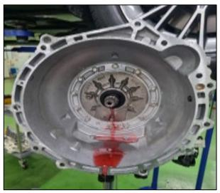
4. Install the new torque converter (B).
